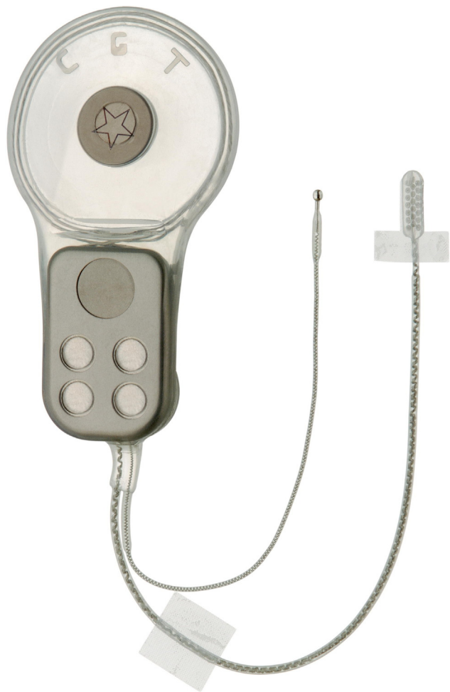
Figure 1 Nucleus auditory brainstem implant. (Color version of figure is available online.)
