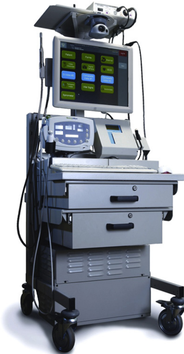
Fig. 1. A telemedicine cart used to collect information during a patient encounter for later review by a remote otolaryngologist using store-and-forward telemedicine. (Image Courtesy of the Alaska Native Tribal Health Consortium, Anchorage (AK); with permission. )
