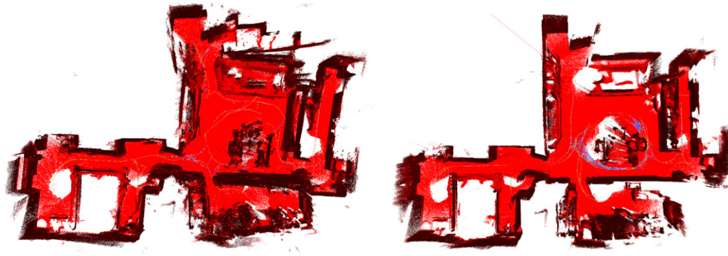
Fig. 1. 3D reconstruction of a home environment from depth data acquired with an ASUS Xtion mounted on a Turtlebot mobile robot. Left: the result using uncalibrated data. Right: the output of the same algorithm when using data calibrated with our procedure. The systematic error in the calibration resulted in noisy open loop estimates that result visible even with correct loop closings.
