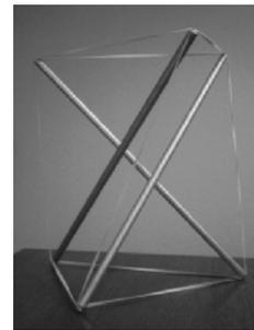
Fig. 1. Example of tensegrity structure.
