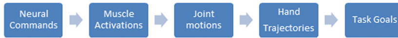
Fig. 1. An illustration of the motor hierarchy: The configuration of each level of the hierarchy uniquely determines the state of the level below (many-to-one). In the other direction, for each configuration in one space there are infinitely many configurations in the space above which satisfy it.
