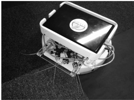
Fig. 2. CrunchBot, a whiskered mobile robot platform.
