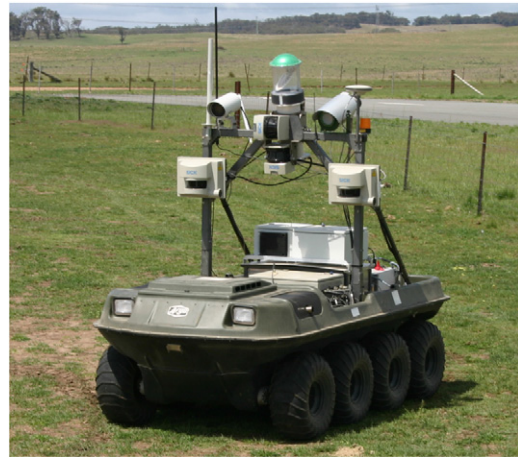
Fig. 1. The CORD UGV employed in this research. The sensor suite is visible, attached to a rigid frame.
