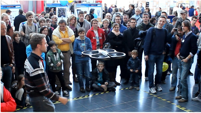
Fig. 1. A low-cost quadcopter navigates in unstructured environments using the front camera as its main sensor. The quadcopter is able to hold a position, fly figures with absolute scale, and recover from temporary tracking loss. Picture taken at the TUM open day.
