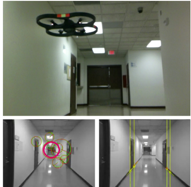
Fig. 1. We use vistas (bottom left) to steer the robot and rely on a map of Wall-Floor Features (bottom right) in a parallel tracking and mapping framework to infer the scene structure and avoid lateral collisions. We present our results in an indoor setting using an AR.Drone (top).
