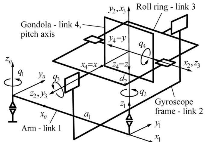
Fig. 2. Coordinate frames of the 4-axis SDT.
