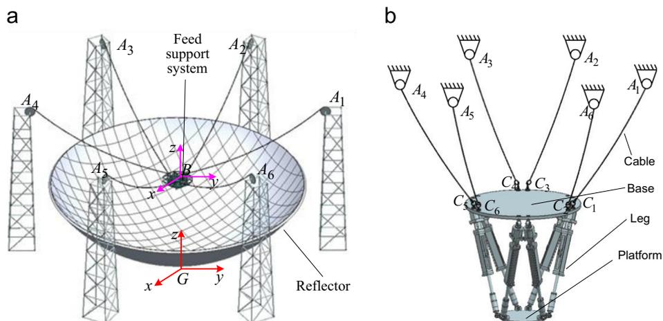
Fig. 1. 3-D model of FAST: (a) isometric view, (b) feed support system.
