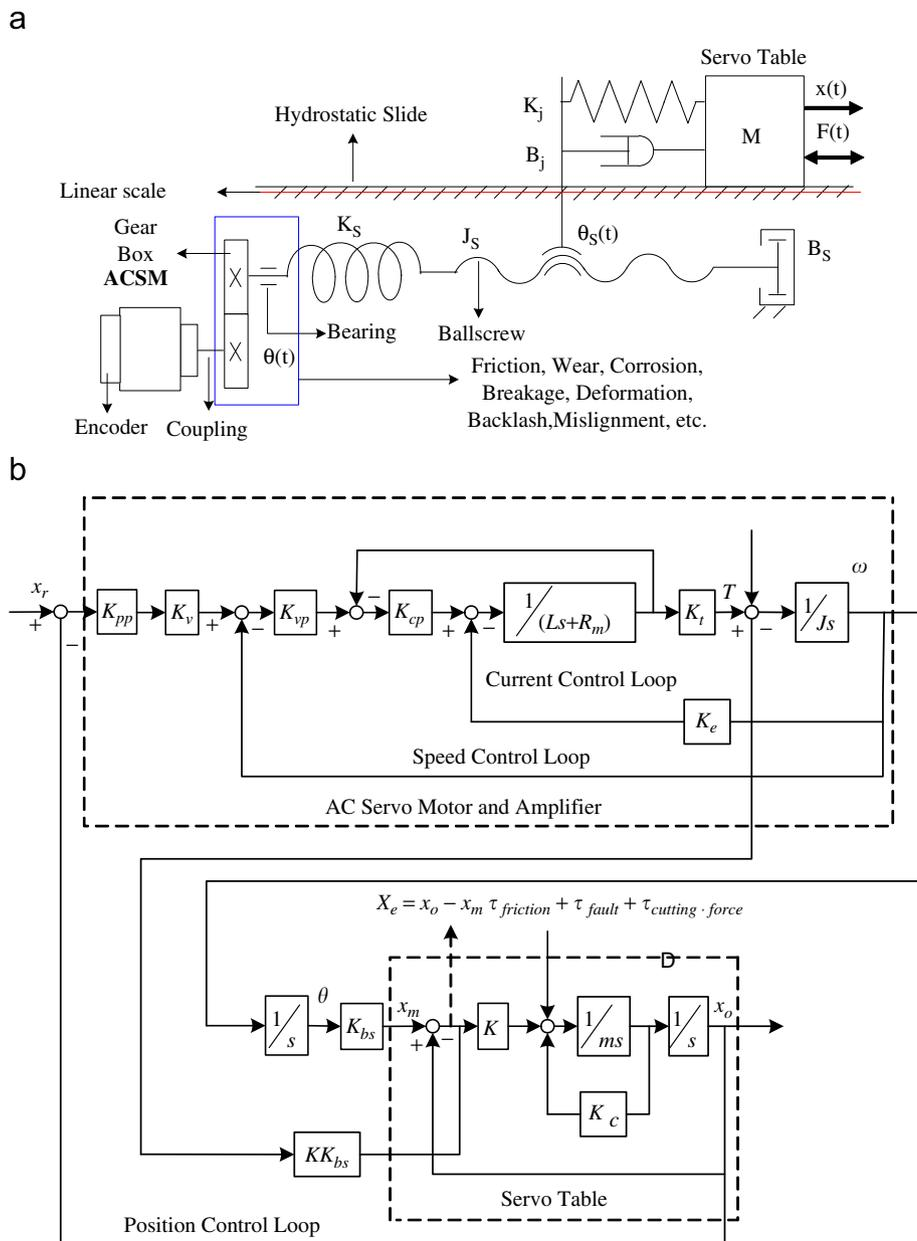
Fig. 1. Mechanical and control system design of machine tool: (a) mechanical configuration of feed drives; (b) block diagram of the servo system.
