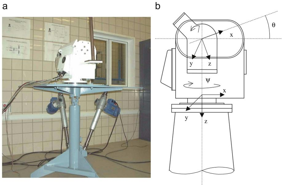
Fig. 1. Two degree-of-freedom platform. (a) Picture; (b) scheme.
