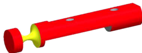
Fig. 3. Right circular multi-axis flexible hinge.
