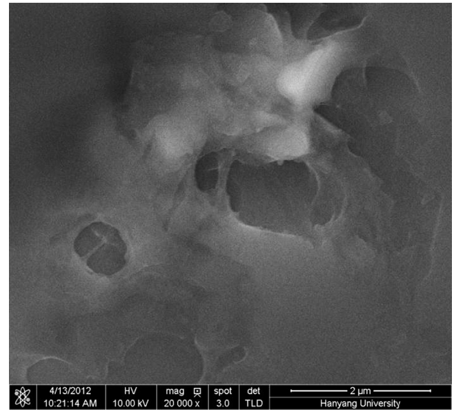
Fig. 1. SEM image of AR-coated surface. The SiO 2 particles are nanosized, so the structure of the AR films during curing varies according to the arrangement of particles. Therefore, process conditions such as the solid content and dry atmosphere are important for improving the transmittance through the formation of a uniform thin film.
