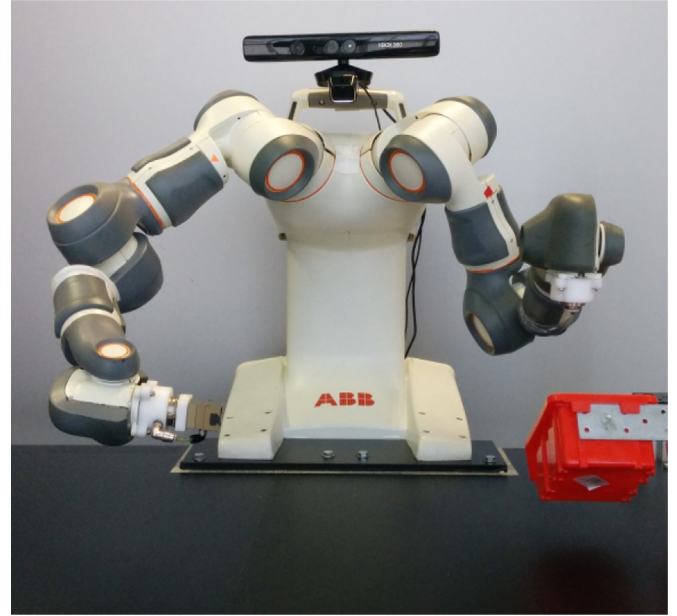
Fig. 1. ABB prototype robot FRIDA. The picture also shows the experimental setup for Experiment #1 and Experiment #2.
