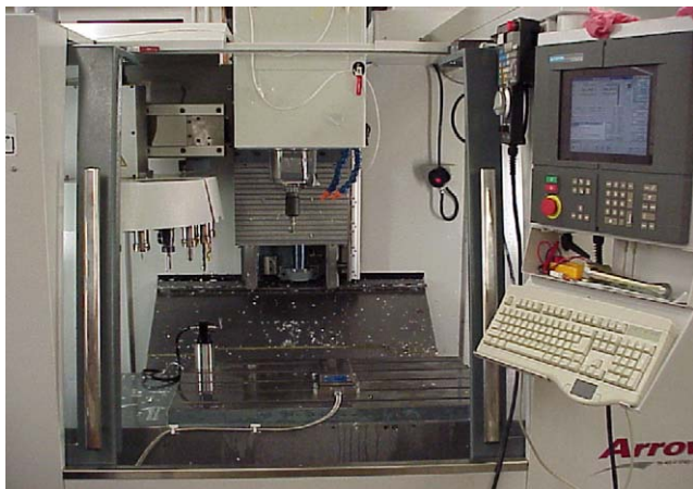
Fig. 1. Experimental setup showing the table mounted Kistler force dynamometer and the spindle housing mounted Kistler accelerometer.
