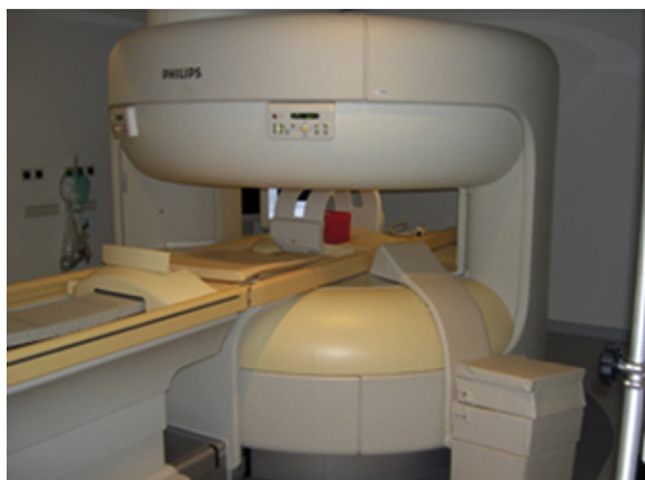
Fig. 1. Experimental set-up in the Panorama open high-field MRI. Shown are the interventional seat at the curvature of the scanner and the phantom in the abdominal coil.
