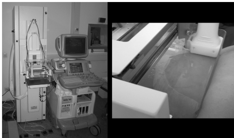
Fig. 1. Prototype of an automated US breast scanner for 3D imaging. There is a Senograph 600 T with a two-axis positioning table and a compression plate on the left and a Logiq 9 US system. On the right the linear M12L probe is mounted on the two-axis positioning table and being used to scan (GE Healthcare, Waukesha, WI).
