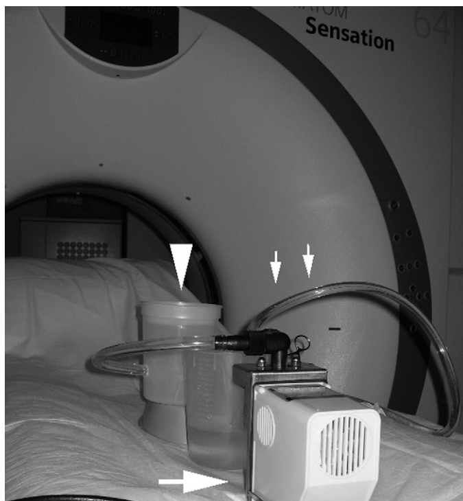
Figure 1. Phantom pulsation was achieved by creating a closed-circuit loop that circulated diluted contrast material via a polyvinyl tube (small arrows) from a blower pump (large arrow) to the aneurysm phantom suspended in a water-filled container (arrowhead). There was continuous pulsation of the aneurysm model during image acquisition.
