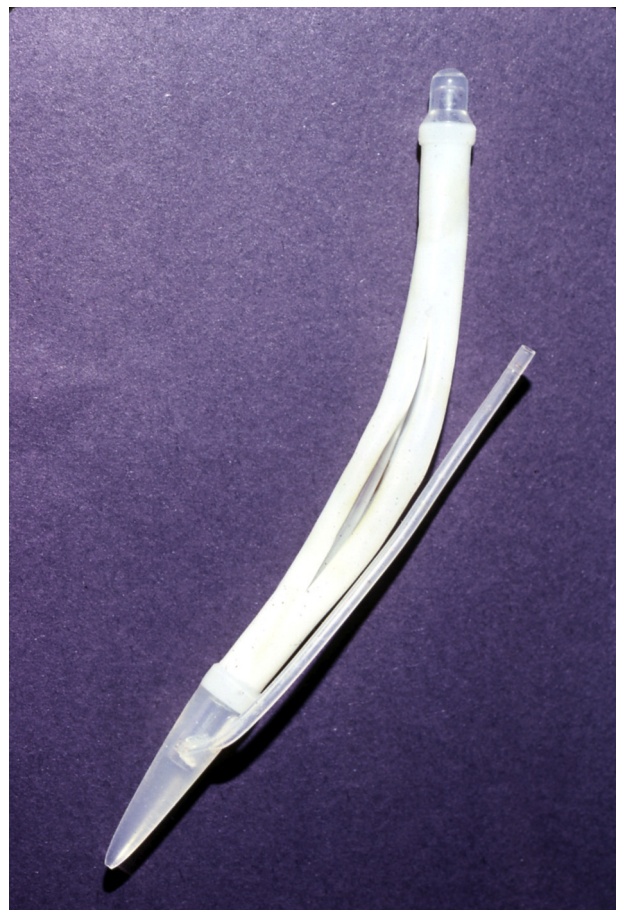
Figure 4. The reinforcing rod against the silicone cylinder caused wear and a defect in the cylinder wall. Figure 4 is available in color online at www.smr.jsexmed.org .
