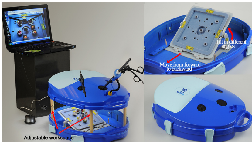
FIGURE 1. Ergo-Lap simulator: The Ergo-Lap simulator ready for use (left); the flexible arrangement of the task panel allows for ergonomic training conditions (upper right); the Ergo-Lap simulator ready for transportation (bottom right).
