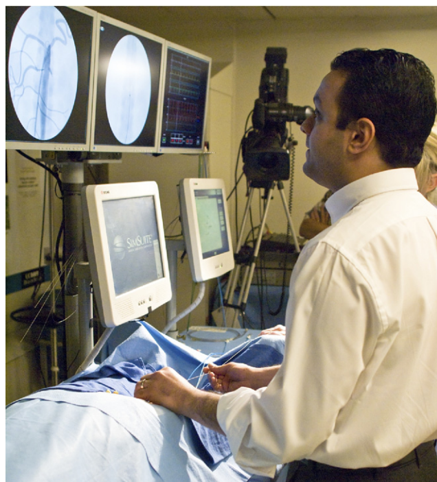
FIGURE 1. Endovascular procedure simulator, demonstrated here with videotape recording for ongoing validation studies.
