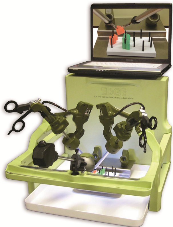
Fig. 1 – The EDGE Platform was developed by Simulab Corporation and is based on a mechanism developed by the University of Washington Biorobotics laboratory. It consists of a pair of interchangeable surgical tools whose motion is constrained to rotate about a fulcrum the same way laparoscopic instruments are constrained by their access ports. (Color version of figure is available online.)
