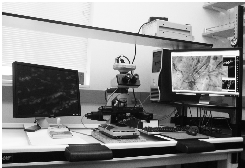
Fig. 1. Photograph of the NeuroLucida tracing workstation. From left to right: (a) the Dell LCD monitor that displays the Lucivid (image plus CRT overlay, not in use); (b) stage-controlling joystick; (c) microscope with Lucivid CRT mounted behind the trinocular head and the camera mounted above the head; (d) the Dell LCD monitor that displays the camera images; a trace is in progress.
