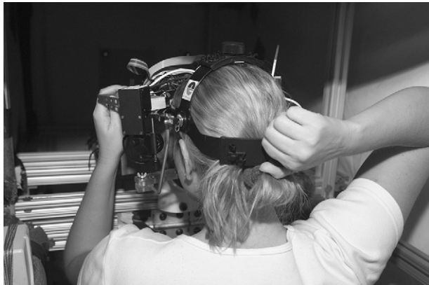
Fig. 1. Binocular video eye tracker (Chronos Vision GmbH). Two side-mounted infrared cameras record eye movements via infrared-reflective mirrors mounted in front of the eyes. A bitebar is used to reduce movement of the headset relative to the head, although movement still occurs.
