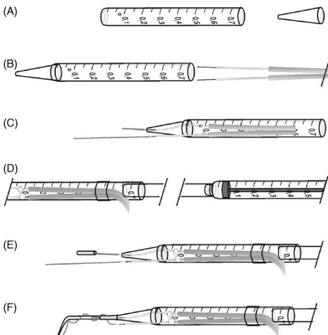
Fig. 1. Steps in the assembly of a suction electrode. See electrode construction in Section 2 for details.
