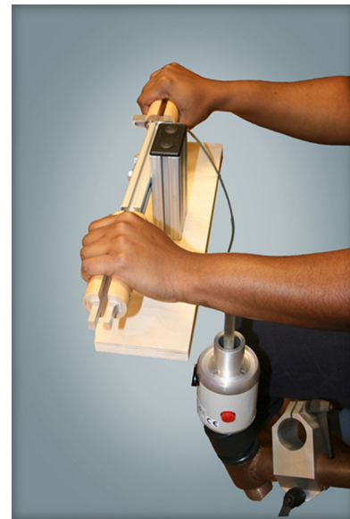
Fig. 1. Custom-designed grasp devices. Composed of a split aluminum force transducer embedded with strain gauges and equipped with semi-circular wooden handles (radius 4.0 cm, length 13 cm). The devices were held horizontally by a coupling support fixed to the table. Right hand flexor muscle vibration case illustrated.
