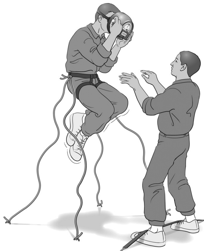
Fig. 1. Artist’s drawing illustrating the goggle device and its use within the aircraft. Note the knob and the readout on the goggle device. The tethers between the subjects’ waist and the aircraft floor were used as a safety precaution to prevent them from drifting away from the operator, who was firmly anchored to the aircraft floor. Drawing Philippe Tausin, SCOM, Toulouse (France).
