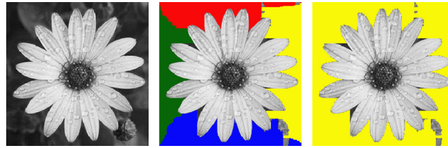
Fig. 1. Image segmentation via k base-line MWRP proposed in [4]. We first convert a picture to a gray scale image. Next, with some suitable function, we construct a pixel grid in which each dark pixel has positive weight and each light pixel has negative weight. Finally we solve the k base-line MWRP to segment the background from the objects. In this example, the boundary edges of the picture are used as base-lines (thus k = 4 ). For example, the red region in the third figure has the top edge of the image as its base-line. (For interpretation of the references to color in this figure legend, the reader is referred to the web version of this article.)
