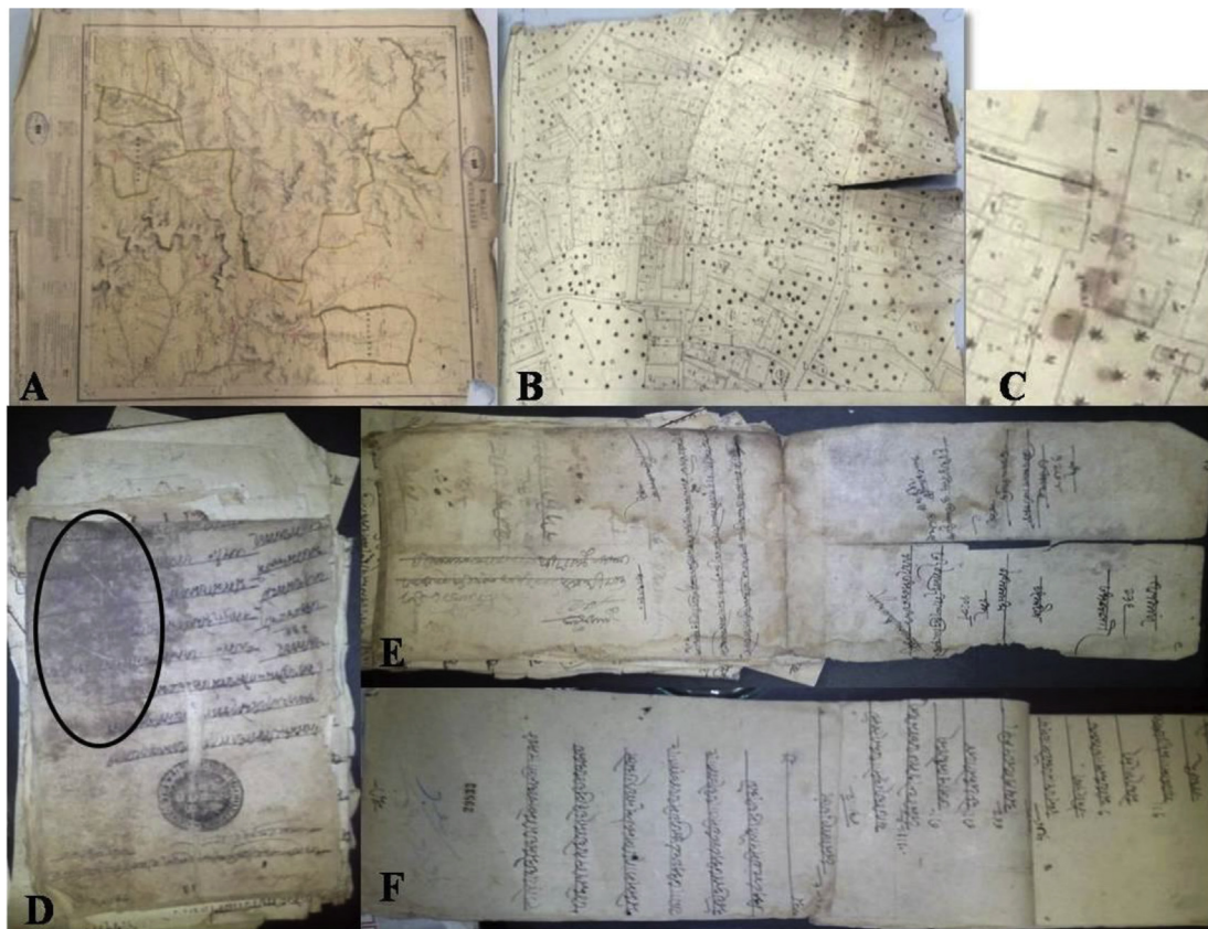
Fig. 1. Some Archival Documents selected for the study (A) Well preserved archival map (B) Foxed tattered brittle archival map (C) Zoomed Foxed area of map from B (D) Stained, foxed daptar (E) Foxed, stained, brittle, torn daptar (F) Well preserved daptar. (samples were procured from the Maharashtra state archives, Mumbai).
