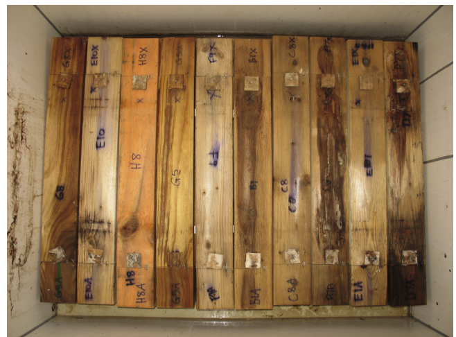
Fig. 1. Samples in an enclosed tank test. The decay feeder block at the far end was Antrodia xantha , while at the near end it was infected with O. placenta .
