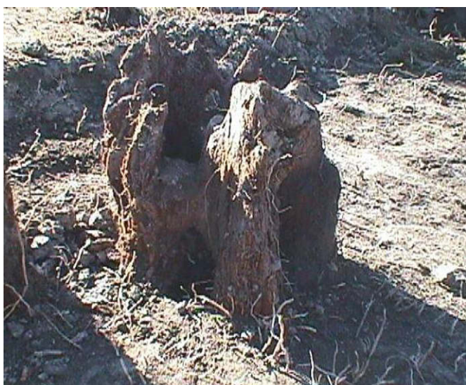
Fig. 2. Wooden pile, exposed to drying.
