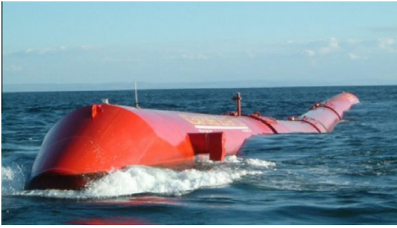
Fig. 1. The Pelamis machine, designed and developed by Ocean Power Delivery Ltd, UK, operating at the Aguçadoura Wave Park, Portugal.
