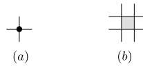
Fig. 1. Vertex drawn as (i) a grid point; or (ii) a unit grid square.
