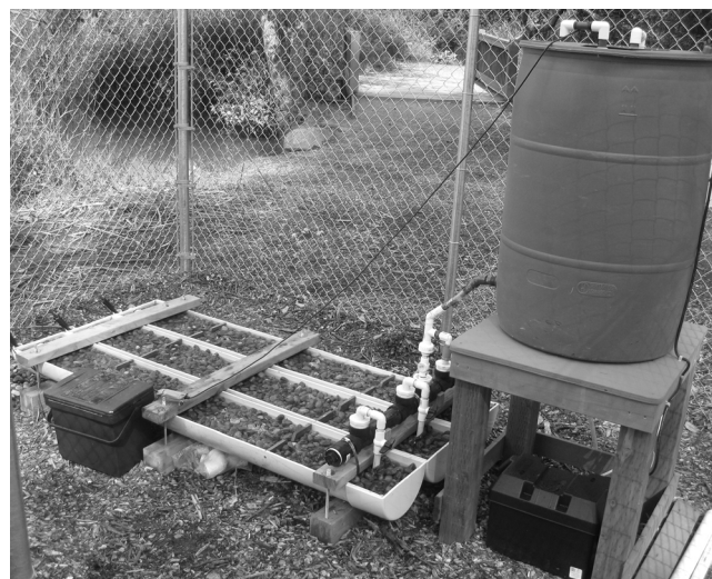
Fig. 1. Rock biofilter system at the beginning of startup with DeCoursey Pond outlet and Clarks Creek in background. Water was pumped intermittently from the pond to an elevated storage tank (to right) and then discharged continuously by gravity to triplicate biofilters. Water moved from right to left through three cells in each biofilter to an outlet pipe. The black case under the storage tank housed a marine battery used to power a submerged pump at the pond outlet.
