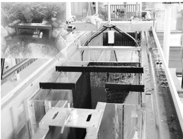
Fig. 2. Experimental GPT rig (50% scale model) placed inside the flume. Fishing net installed downstream at end of raceway capturing exiting spheres. Top left, a view of the GPT LitterBank in situ with high downstream tidal waters.
