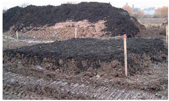
Fig. 1. Experimental setup at Bidston demonstrating the incorporation of compost with the other soil forming materials.
