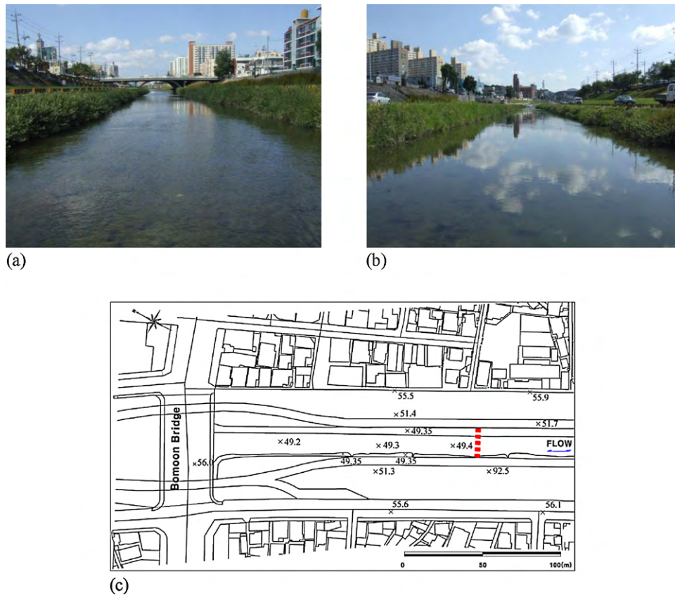
Fig. 1. Photo of the study reach and topographic reach map of the Daejeon Stream. (a) Photo of straight trapezoidal reach looking upstream. (b) Photo of straight trapezoidal reach looking downstream. (c) Topographic reach map.
