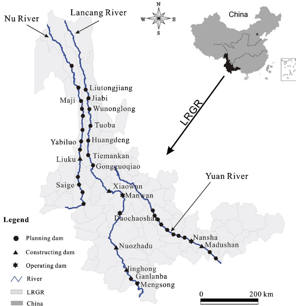
Fig. 1. Distribution of dams on mainstems of Lancang River, Nu River and Yuan River in LRGR.
