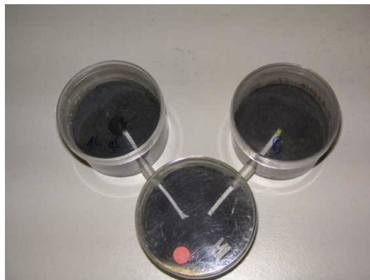
Fig. 1. Dual choice olfactometer design. Three plastic vessels (Ø 5 cm, height 3 cm, filled with Plaster of Paris layer) were connected via two silicon tubes. For eased passage from the starting chamber (indicated with a red dot) into the choice chamber, moist filter paper was laid though the tubes. Choice chambers were provided according to experiment 1 and 2. (For interpretation of the references to colour in this figure legend, the reader is referred to the web version of this article.)
