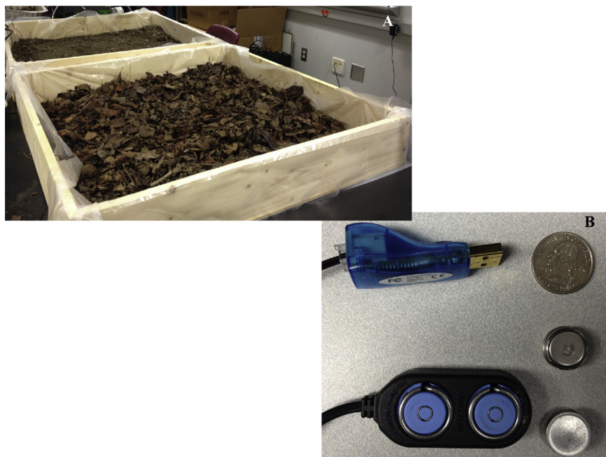
Fig. 1. The microcosm experimental setup (A) and a photo of iButtons and iButton data reader (B). The US quarter is for scale.
