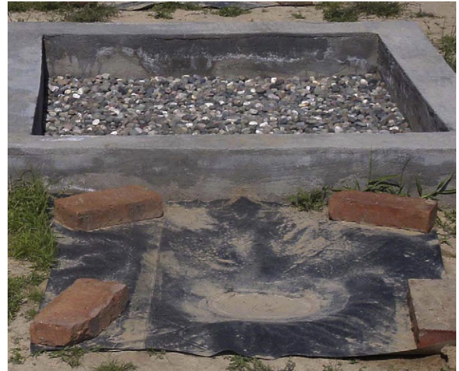
Fig. 1. Concrete bordered plots (1 × 1 m) for measuring runoff and soil water content; the plot contains 10 cm thick pebbles, the black plastic sheet covering the barrel is used to prevent catching precipitation and evaporation of the collected runoff water.
