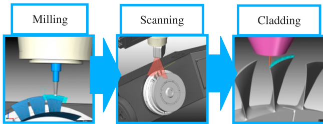
Fig. 1. Process chain for the repair of a damaged turbine blade.
