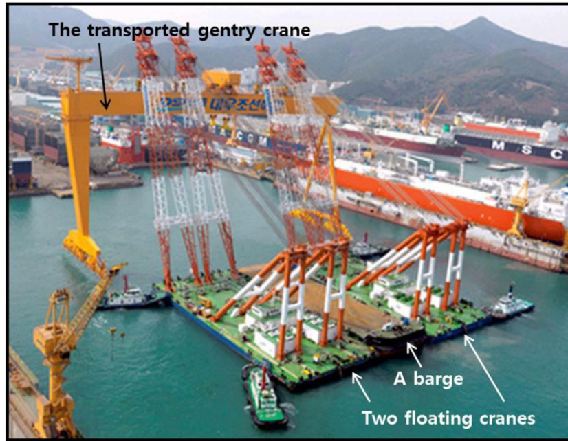
Fig. 1. Transportation of the gantry crane using parallel connected floating cranes and a barge in DSME (Daewoo Shipbuilding and Marine Engineering, Co., Ltd.)
