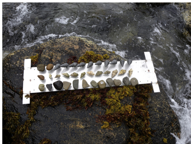
Fig. 2. One of the metal frames with the three substrate types prior to deployment on the sea bed.
