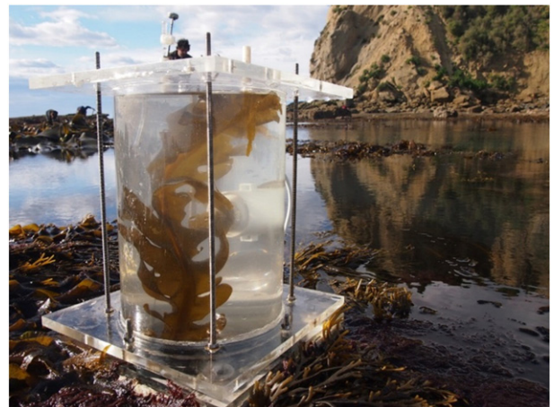
Fig. 1. In situ photorespirometry chamber fitted around a macroalgal assemblage, dominated by Undaria pinnatifida at 'The Point' Moeraki, New Zealand.
