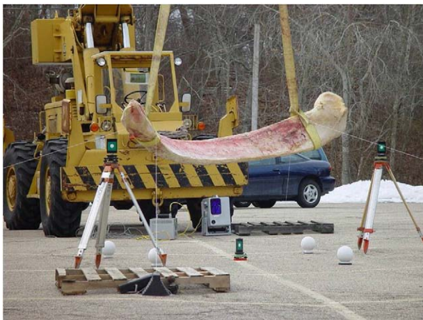
Fig. 1. 3-D laser scanning of the mandible at the Woods Hole Oceanographic Institution (MA, USA) to determine the surface geometry.
