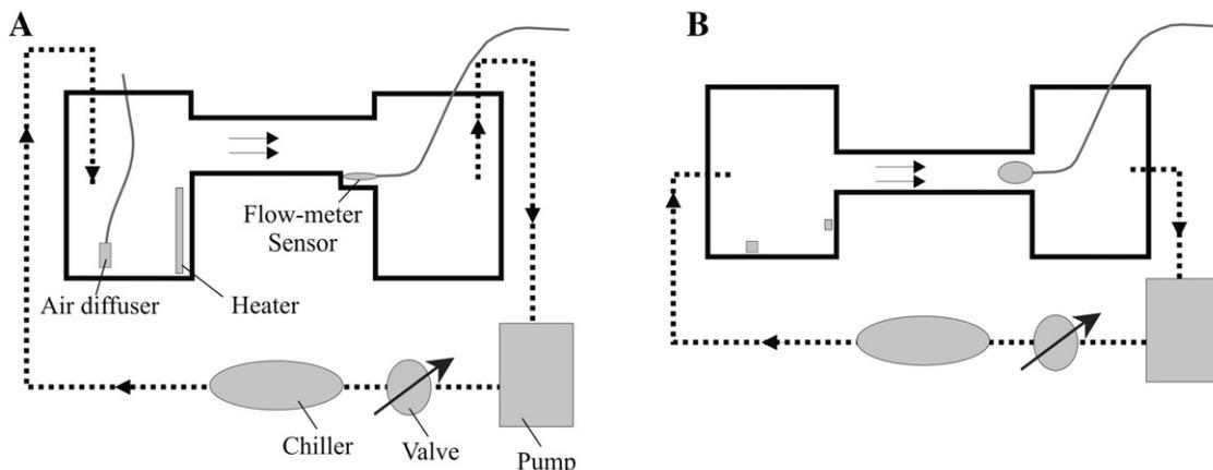
Fig. 1. Swimming apparatus used in the present study. (A) Lateral view; (B) top view. Arrows indicate the direction of water circulation.
