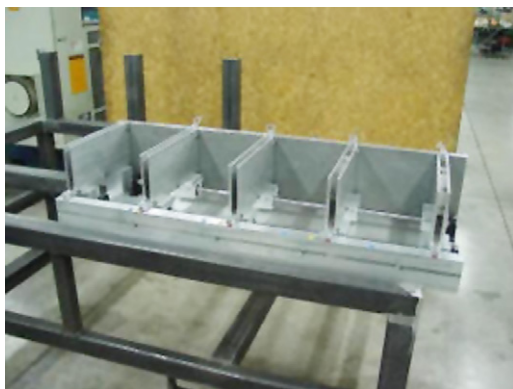
Fig. 4. Assembly fixture to locate shelves for assembly of cabinets (pioneer industrial systems LLC.) [21].
